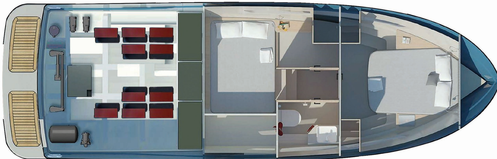
Lower Deck 2 engines - 2 x Steerable POD Electric Engine
